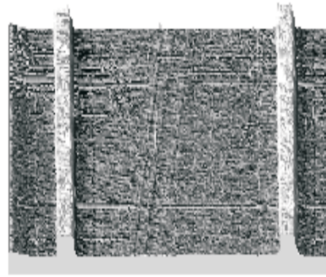
Fig. 2. Atomic force microscopy picture of the Co/CoO wire structures. The period of the parallel wire structure is equal to 15\ \mu\text{m} .
